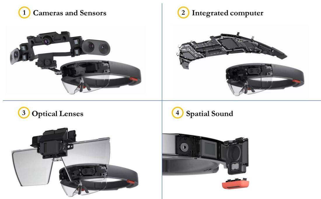
Figure 3.11: HoloLens's Modules [10]
