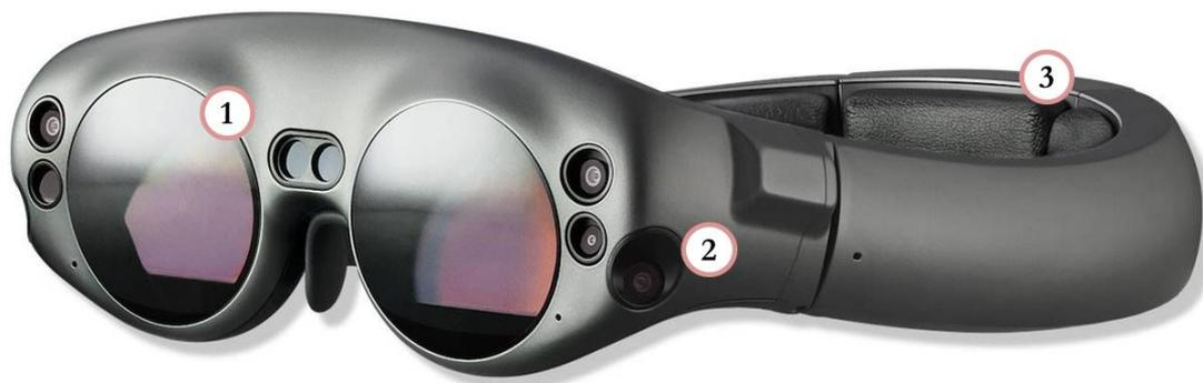
Figure 3.13: Magic Leap One. (1) Optical Lenses (2) Cameras and Sensors (3) Spatial Sound
